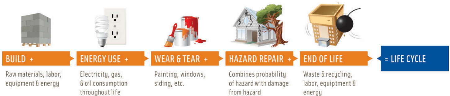
FIG. 5. Quantifying the impacts for all phases throughout a building's life is accomplished through a life cycle cost analysis.
